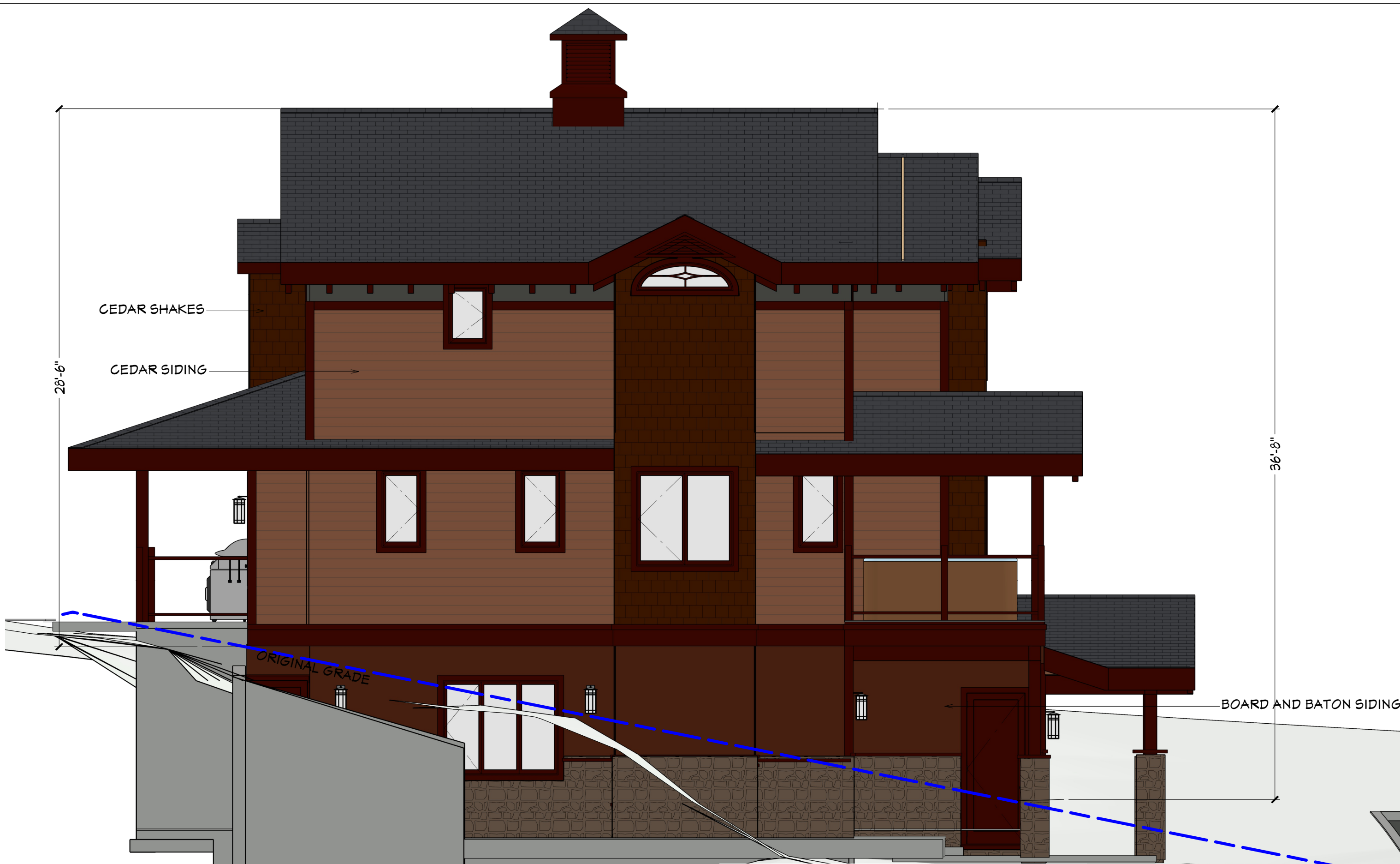
Left Elevation Average Height 32'7" or 9.9m
